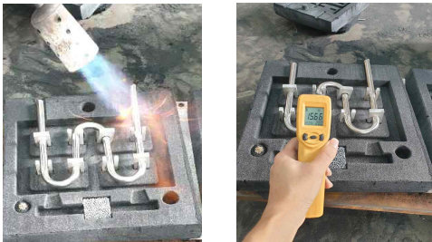
Fig. 7 Sand Mold Assembly (Check the temperature of the insert part)
