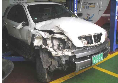
Fig. 1 The front right side of Sorento is collapsed
