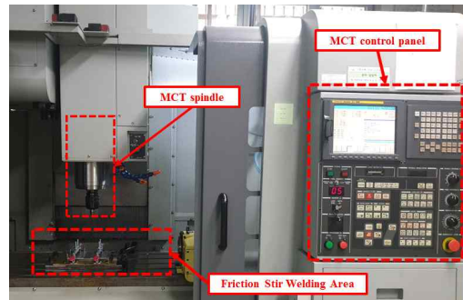
Fig. 1 Friction stir welding experiment device
