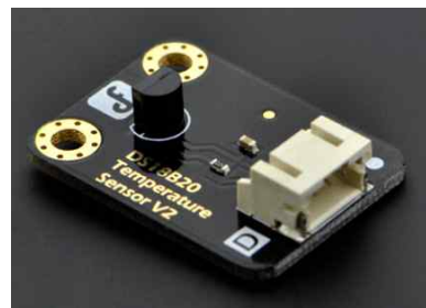
Fig. 6 Temperature sensor DFR0024 module
