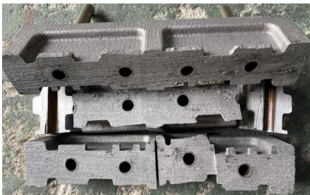
Fig. 12 Visual inspection of internal pores
