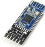
(b) HM-10 (bluetooth data transmission module)
